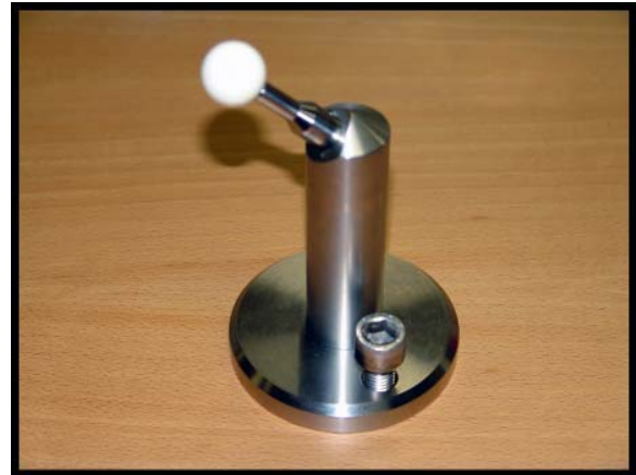
Sphere, Mounting Base, and M12 Screw
